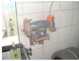
Grinding wheels with the protective covers removed.
