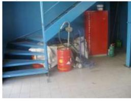
Storage of combustible materials (in this case flammable) under a staircase, not to mention the installation of a Fire Hose as well as other fire-fighting equipment in a semi-accessible area.
