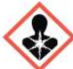
Serious health hazard
